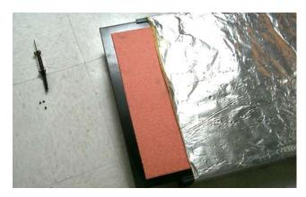
Fig. 12: The heater plate slides from the insulation.
